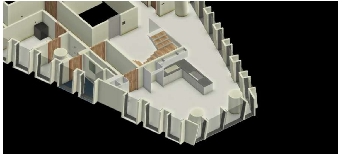
Point Cloud model Converted to BIM from Point cloud model in Riyadh, Saudi Arabia
