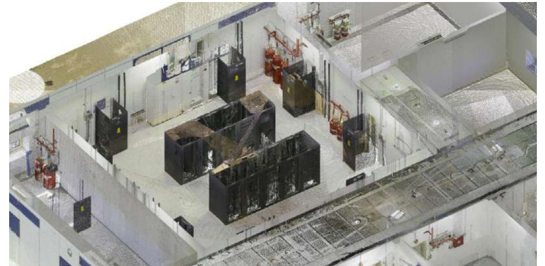
Point Cloud model for Scan To BIM Project in Riyadh, Saudi Arabia
